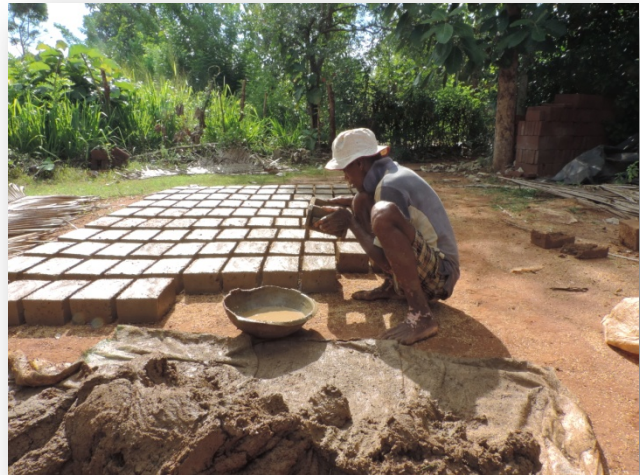
Fig 5.3.1 Dharmaratne making bricks with rice husk brick mixture
