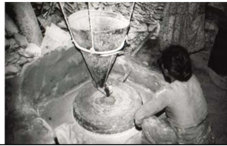
Figure: Improved Water Mill for Multiple Application (Sketch on the left and photo of Operation for Grinding on the right)
