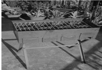
Honeycomb briquettes used inside a barbeque unit with air-intake regulators
